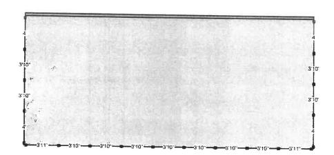
Dimensions are measured from the center of each railing post.
